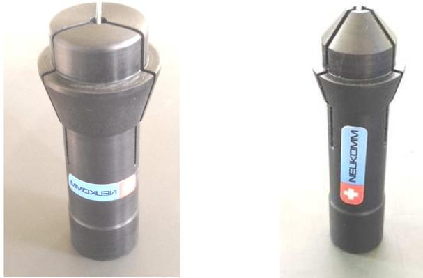
**The polymer collet does not mark, nor scratch the bar or the part at clamping.**
